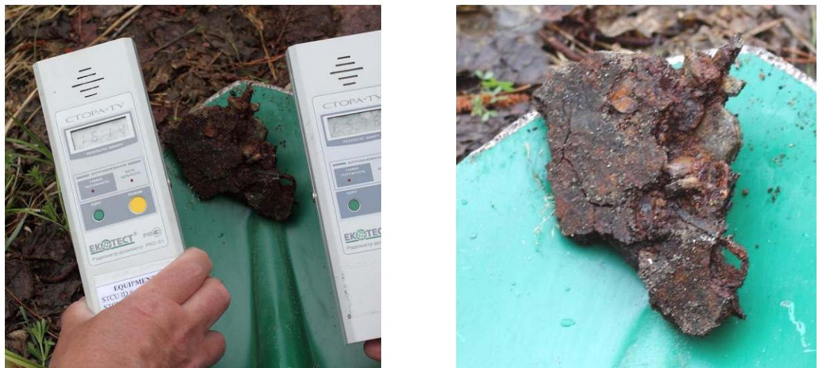
Fig. 1.11. Fragment of ferroconcrete construction with PED and density of beta flow exceeding the blank meanings up to three order of magnitude.
