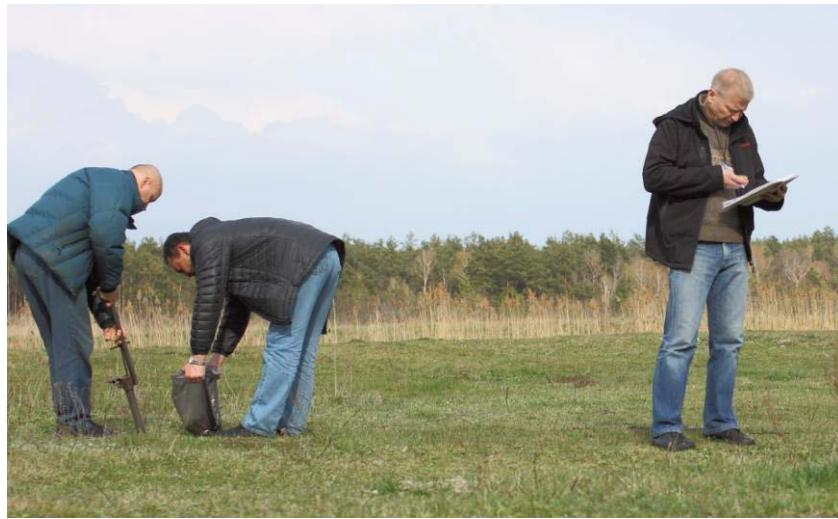
Fig. 1.7. Procedure of soil sampling.
