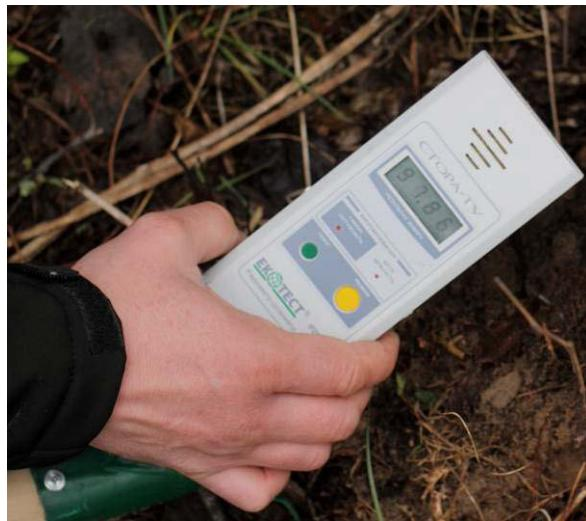
Fig. 1.10. Detection of the local source of radioactive contamination with high meaning of PED
