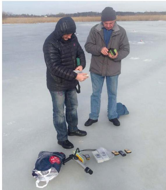
Fig. 1.5. Measurements of zero background for dosimeters on ice over the water body.
